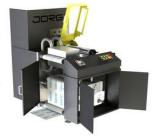
The JORG ILP.330 Inline Priming Unit can be easily connected between the unwinder and the main unit (printing unit) of an HP Indigo ws4xxx and 6xxx web press.
