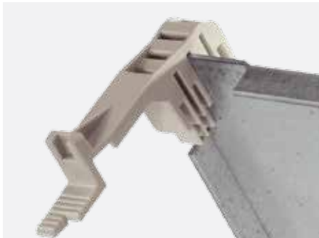
The fixing hooks and feet supplied in the standard versions are applied without having to use tools, making it possible to install the base plate at seven different depths inside the switchboard. They can also be adjusted at three further positions.
