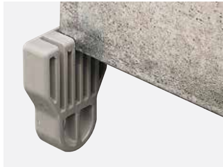
The fixing hooks and feet supplied in the standard versions are applied without having to use tools, making it possible to install the base plate at seven different depths inside the switchboard. They can also be adjusted at three further positions.
