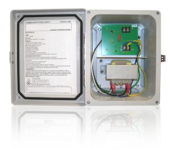
The PWR-24AC-1-3-ULW is a CCTV power center engineered to manage remote camera and accessory power requirements in a NEMA 4X weatherproof enclosure. The PWR-24AC-1-3-ULW distribution module is designed with 1 individually fused output for powering up to 1 CCTV camera or accessory. It will provide 24Volts AC via distribution to one fused output with a total of 3.0 Amps continuous supply current.
